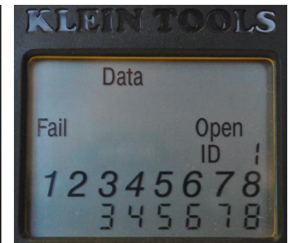
Open Wires – FAIL (pins 1 & 2)
