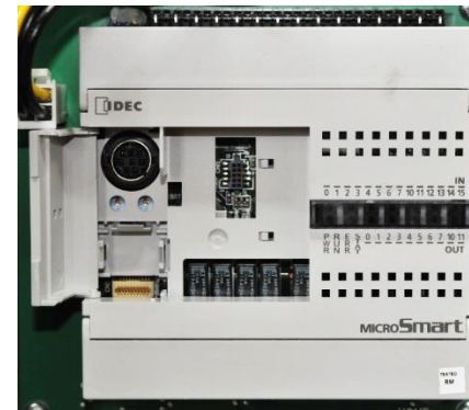
Depress The Tab On the Left and Remove the Cover
