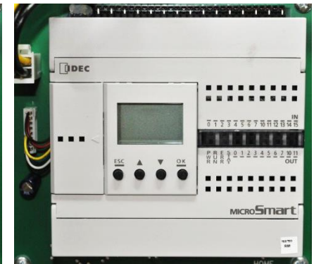
Gently Plug In the LCD and Close the Cover
