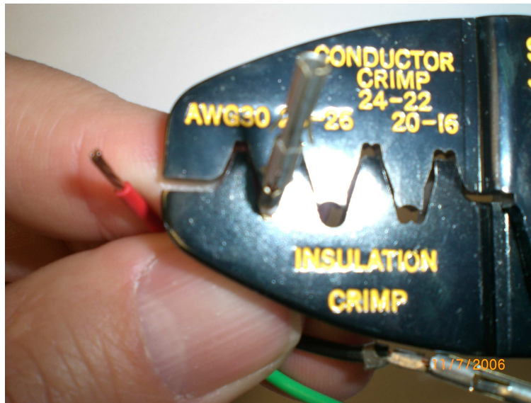
Figure 61 – Crimping Pins onto 18-4 Wires (Female Shown)
