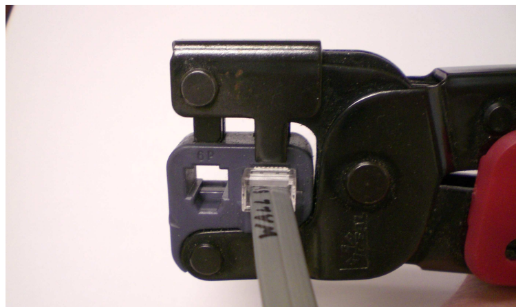
Figure 68 – Crimping RJ45 Connector to 28-8 Cable
