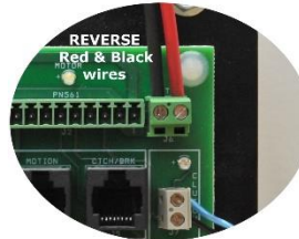
Figure 4 – Reverse Motor Polarity
